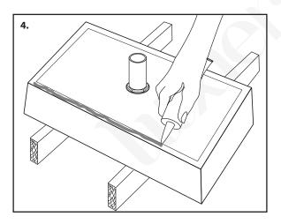
4. Place the assembled vessel sink through the 3 1/2" opening on the counter top and check for level and fit. Plumber's putty can be used to level the sink. Apply silicon adhesive around the bottom rim of the sink as shown.
