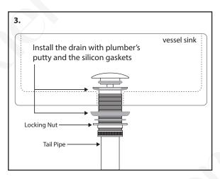
3. Attach the pop up drain to the ceramic sink as shown. It is recommended to use plumber's putty with the silicon gaskets to prevent any possible water leak. Make sure the drain is properly secured to the vessel sink.
